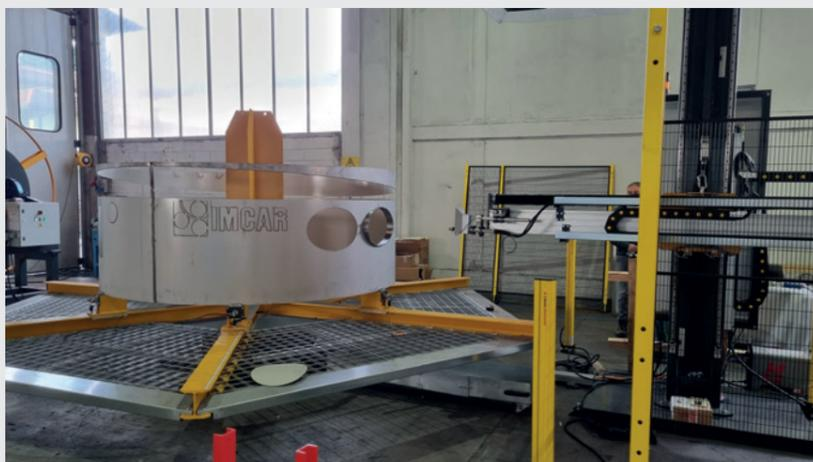
Imcar keeps a constant relationship with its customers also after the sale to provide a steady service, but also to understand customer's needs over time and optimize the various production departments. During these latest years, Imcar has developed a new automated solution, a tank cutting system, able to do all cutting operations for the connection of accessories, like doors and sloping bottoms.
