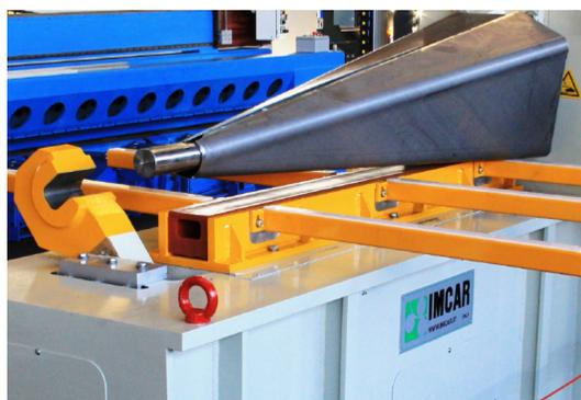
Hydraulic press. The electronic parallelism and the polyurethane covering with stainless steel devices prevent damage to the sheet during the forming process.
