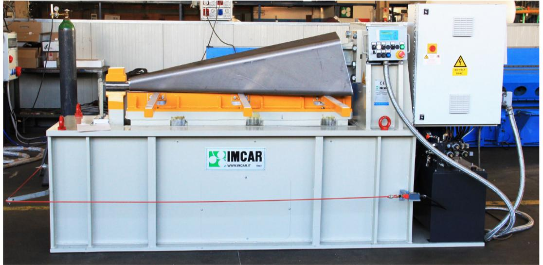
The Imcar press allows to realize the supports for the tanks in four phases, reducing production times and number of welds.
