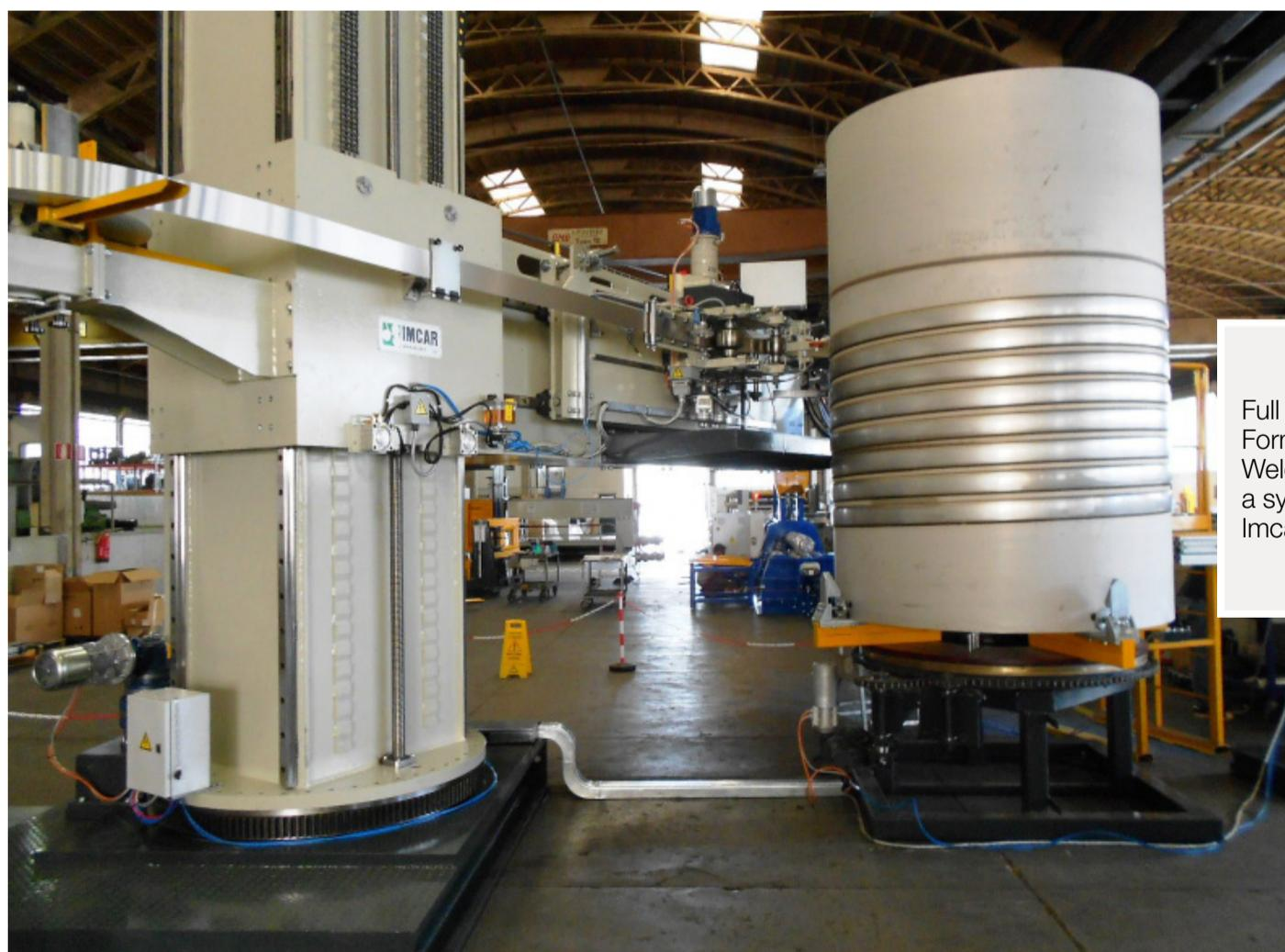
Full Automatic Half Pipe Forming, Bending and Welding Technology, a system designed by Imcar.
