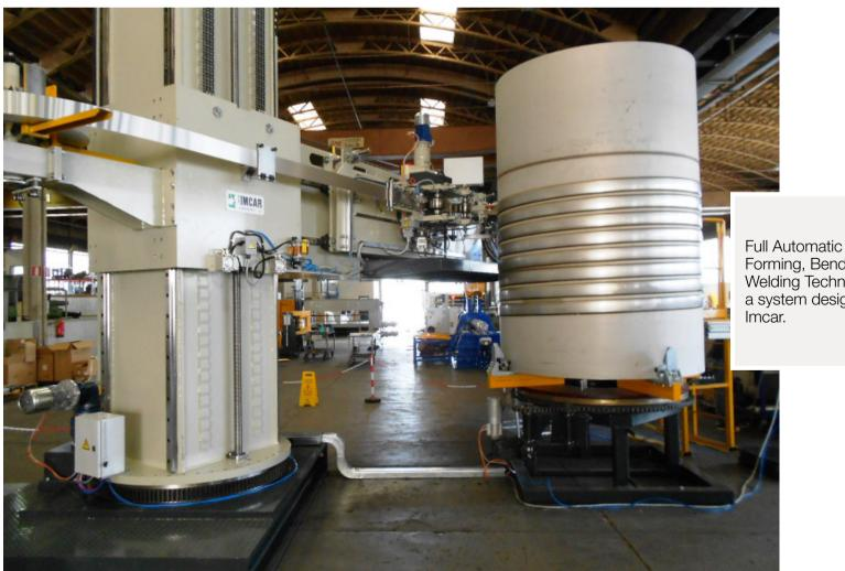
Full Automatic Half Pipe Forming, Bending and Welding Technology, a system designed by
