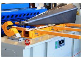
Hydraulic press. The electronic parallelism and the polyurethane covering with stainless steel devices prevent damage to the sheet during the forming process.
